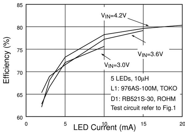
Fig. 10 5 LEDs Efficiency vs. LED Current
