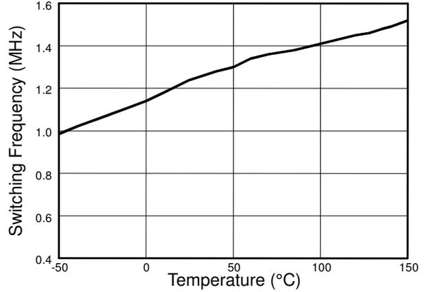
Fig. 3 Switching Frequency vs. Temperature
