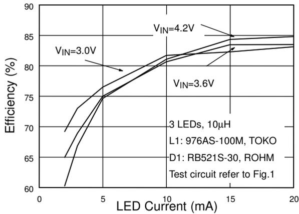
Fig. 8 3 LEDs Efficiency vs. LED Current
