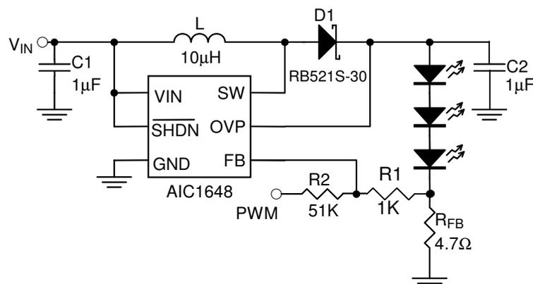
**Fig. 17 Dimming Control Using a PWM Signal**
