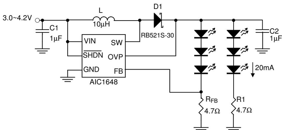
Fig. 20 Six White LEDs Application in Li-Ion Battery
