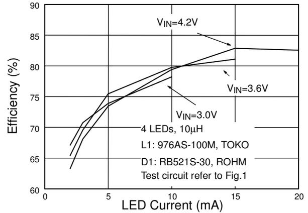
Fig. 9 4 LEDs Efficiency vs. LED Current
