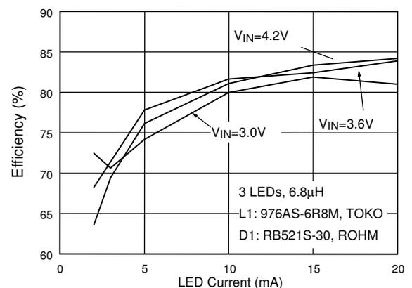
Fig. 1 Li-Ion Powered Driver for Three White LEDs
