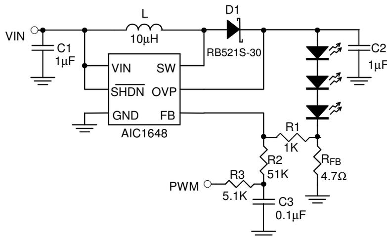
Fig. 19 Dimming Control Using a Filter PWM Signal
