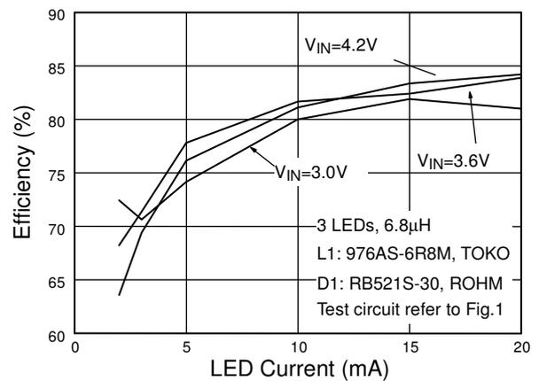
Fig. 11 3 LEDs Efficiency vs. LED Current
