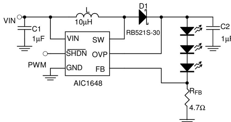
**Fig. 16 Dimming Control with a PWM Signal**
