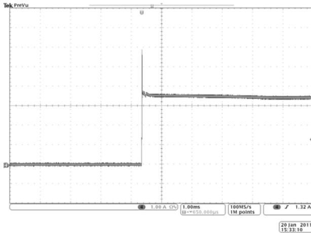
Fig.15  $V_{IN} = 1.8V$ ,  $V_{REF} = 0.9V$  Sink Short Circuit
