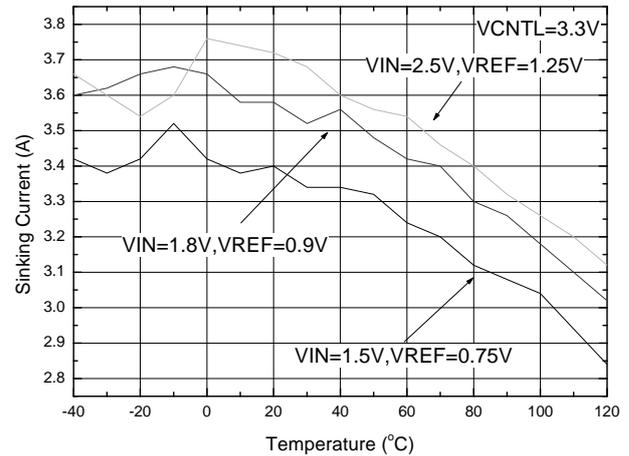
Fig.4 Current limit (Sinking) vs. Temperature
