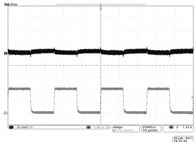
Fig.6  $V_{IN} = 1.8V$ ,  $V_{REF} = 0.9V$  Source Response
