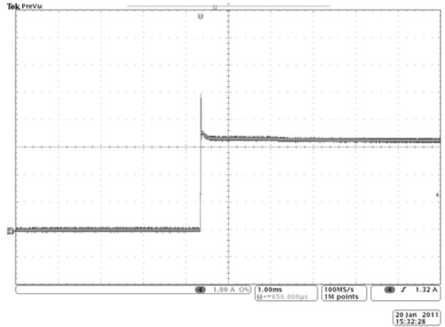
Fig.14  $V_{IN} = 1.5V$ ,  $V_{REF} = 0.75V$  Sink Short Circuit
