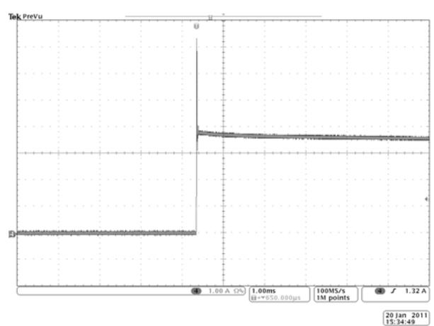
Fig.16  $V_{IN} = 2.5V$ ,  $V_{REF} = 1.25V$  Sink Short Circuit
