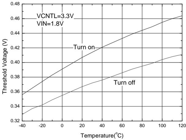
Fig.1 Turn on and turn off vs. Temperature
