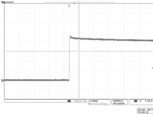
Fig.13  $V_{IN} = 2.5V$ ,  $V_{REF} = 1.25V$  Source Short Circuit
