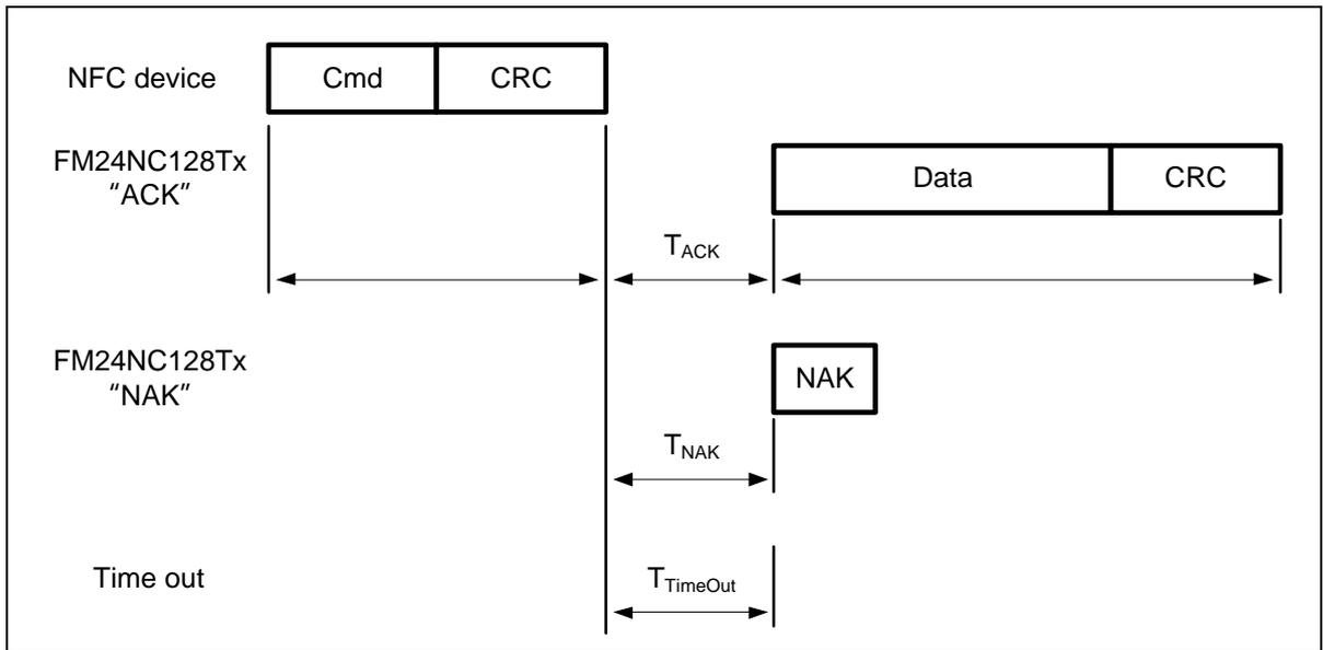
Figure 28 READ\_RF\_DATA\_RD\_LOCK command
