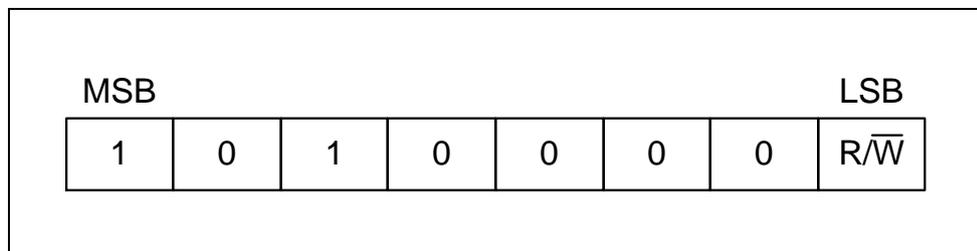
**Figure 8 Device address of two wire serial interface**
