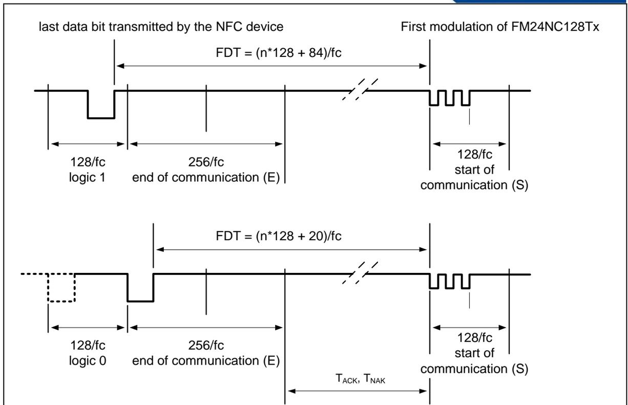
Figure 19 Frame Delay Time (from NFC device to FM24NC128Tx),  $T_{ACK}$  and  $T_{NAK}$
