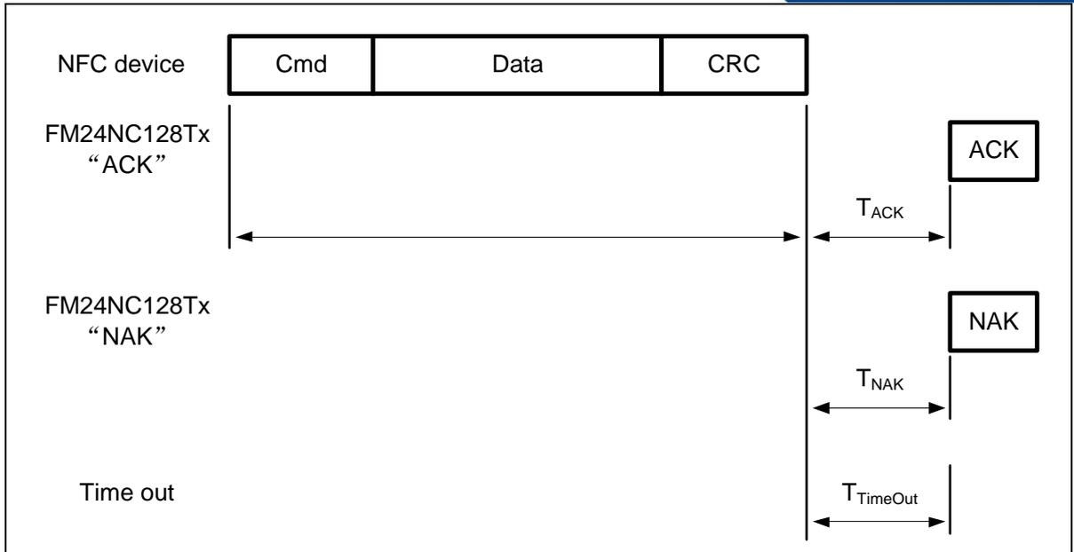
Figure 31 WRITE\_RF\_DATA\_WR\_LOCK command
