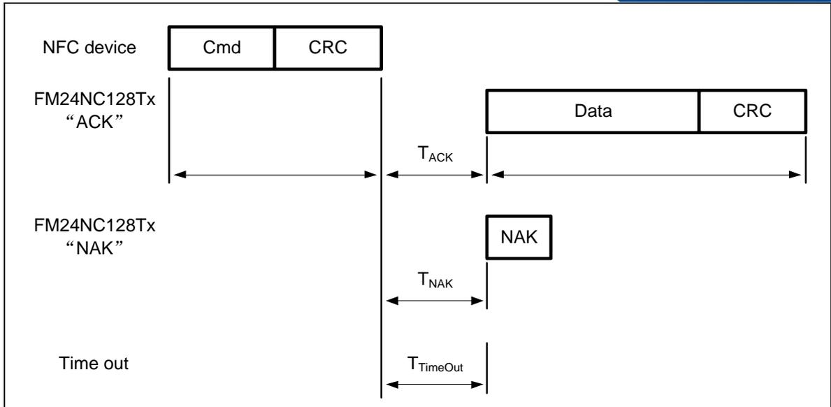
Figure 29 READ\_RF\_DATA\_WR\_LOCK command
