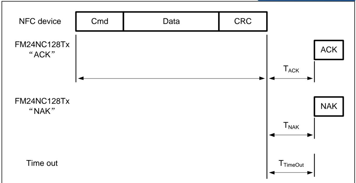
Figure 30 WRITE\_RF\_DATA\_RD\_LOCK command
